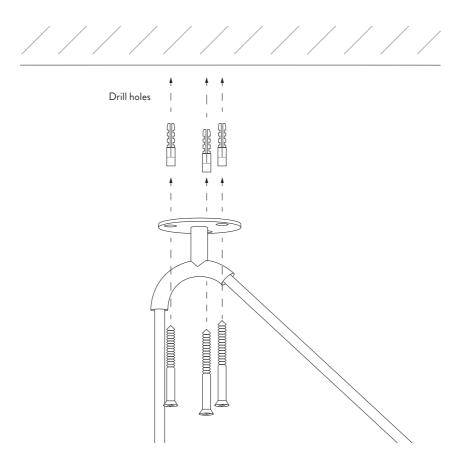
Use the ceiling bracket to mark the three holes  $\acute{p}$  ositions. Drill the holes and insert the rawplugs. Fix the ceiling's bracket thank to the 3 long screws.
