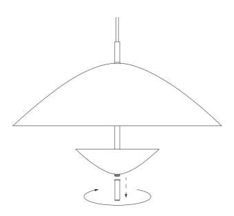
Unscrew the rod at the bottom of the lamp and remove the cover.
