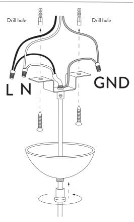
Make connect to the main supply using suitable nuts N. White, L, Black, Green/yellow, GND. Screw the canopy bracket to the junctions box in the ceiling using two screws.
