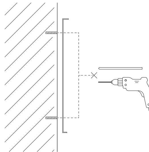
Use the wall mount to mark the two holes with a pencil
