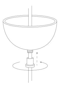
$\label{eq:makeronnect} \textit{Make connect to the main supply using suitable nuts N. White, L, Black, Green/yellow (grey), GND. \\ \textit{Screw the canopy bracket to the junctions box in the ceiling using two screws.}$
